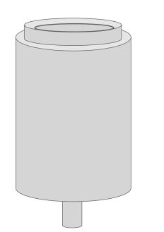
Requires level surface And protection from wind The tipping bucket rain gauge measures rainfall by volume of water that accumulates in a pair of inner cups which alternately fill and drain. Algorithms calculate rain in inches based on number of times the cups were filled and drained.
